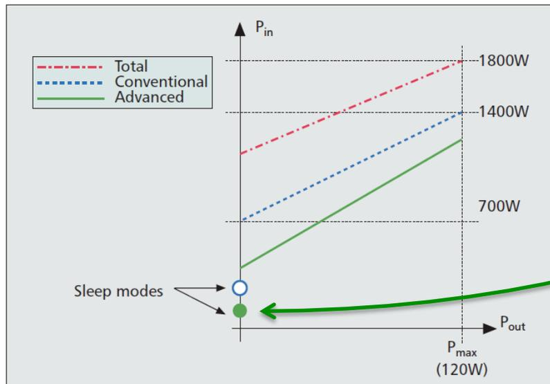
Linear model for a 3-sector macro base station. "Conventional" does not include power supply and cooling.
