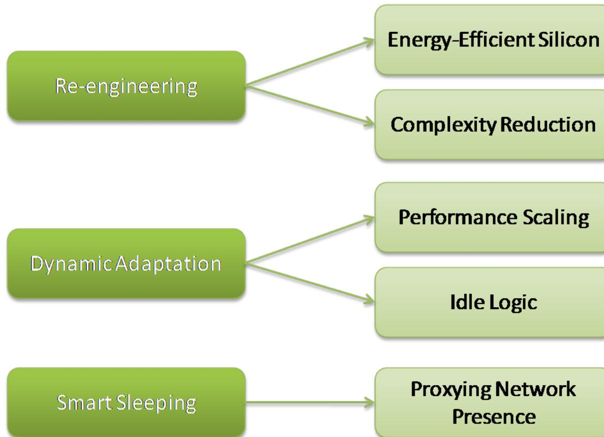
Techniques can be applied at **device**, **link**, and **network** levels. Most of them apply to both wired and wireless.
