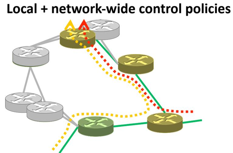
Once network devices will include energy management primitives, further energy reduction will be possible by moving traffic flows among the network nodes, in order to minimize the energy consumption of the entire infrastructure. [This is definitely a point of contact between wired and wireless.](#)
