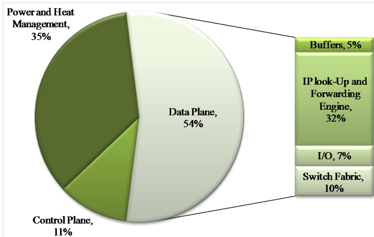
Estimate of power consumption sources in a generic platform of high-end IP router.
