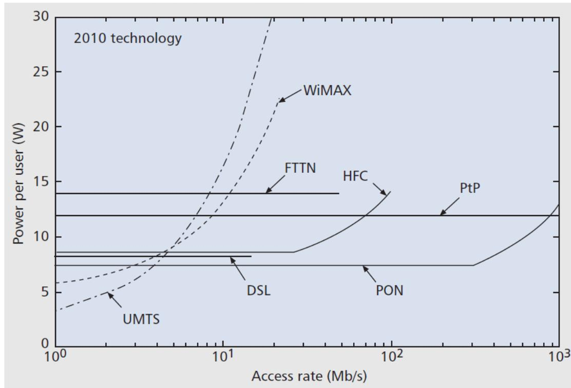
Power consumption of DSL, HFC, PON, FTTN, PtP, WiMAX, and UMTS as a function of access rate with an oversubscription rate of 20. The technology used is fixed at 2010 vintage for all access rates.
