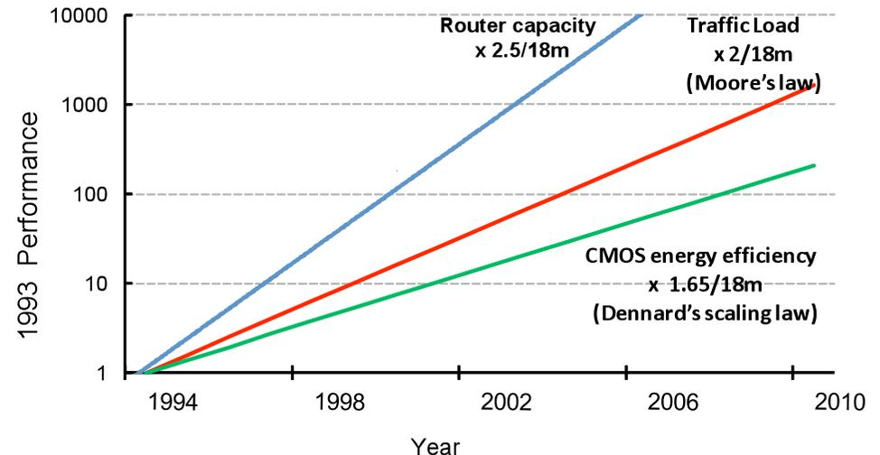
Evolution from 1993 to 2010 of high-end IP routers' capacity (per rack) vs. traffic volumes (Moore's law) and energy efficiency in silicon technologies.
