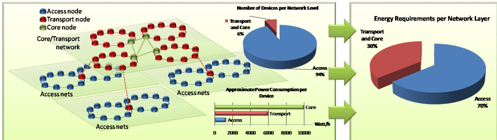
Typical access, metro and core device density and energy requirements in today's typical networks deployed by telcos, and ensuing overall energy requirements of access and metro/core networks.
